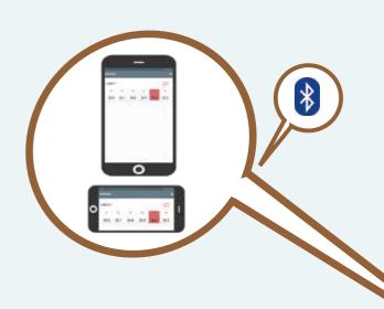
Installing a scanner node, it is possible to access the temperature data remotely from any device connected to the Internet by means of a Web application. The application allows monitoring temperatures in real time as well as displaying graphs with the evolution of temperatures over a certain period. The scanner node can also send a warning via e-mail when the temperature of a point overpasses a certain threshold configured by the user.
